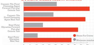
Slip Resistance Test EN ISO 13287:2012, performed by TUV Rheinland LGA Products GmbH in Leipzig, Germany during August 2018\* On a scale where 0.0 is the absence of friction and 1.0 is very high friction (e.g. dry carpet), SFC rated .63 – more than tripling the .18 minimum standard. All SFC shoes use the Shoes For Crews patented slip-resistant outsole. Product tested: BRIDGETOWN 28740
